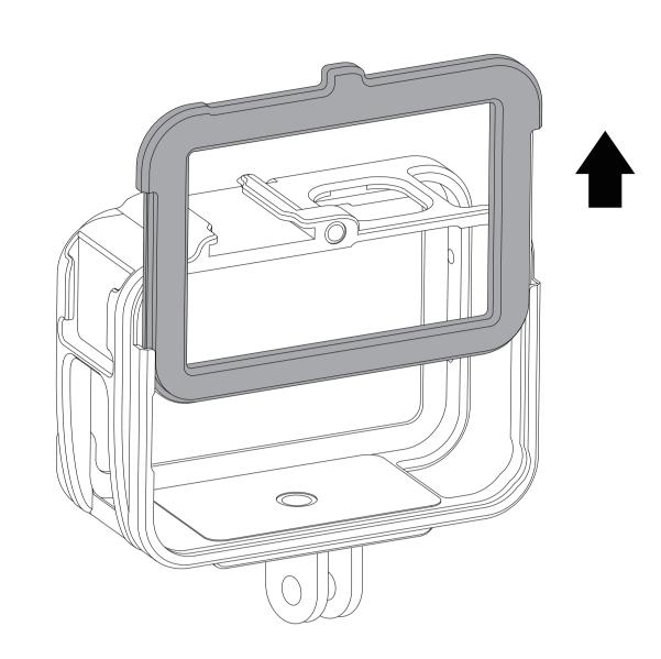
2 Remove the side cover of the sports camera 拆除运动相机侧盖
